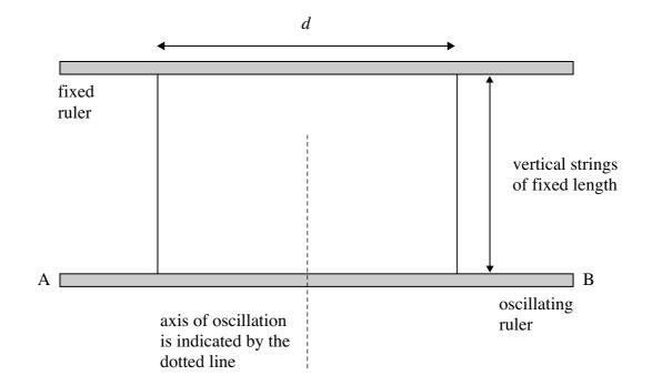
A student conducts an experiment to investigate the relationship between the time period, T, of the suspended oscillating ruler, and the distance, d. The student's results are shown in the table.
