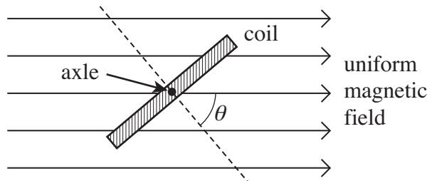
A coil of 50 turns has a cross-sectional area of  $4.2 \times 10^{-3} \text{ m}^2$ . It is placed at an angle to a uniform magnetic field of flux density  $2.8 \times 10^{-2} \text{ T}$ , as shown in the diagram, so that angle  $\theta=50^\circ$ .
