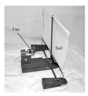
This boat has a solar-powered fan attached. The fan blows air towards the sail.
