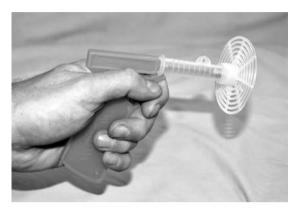
The flygun consists of a handle, a spring and a disc as shown in the photograph below.
