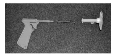
When the trigger is pulled, the compressed spring is released, launching the disc at the fly.
